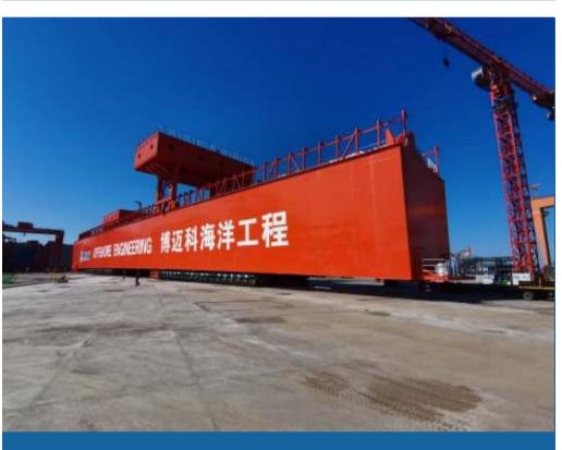
Sarens SPMTs Load-in and Transport Crane in Tianjin, China
